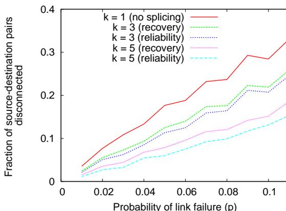
Figure 5: Recovery using *network-based recovery* and Sprint topology.
